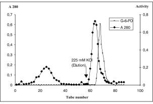
Figure 2. Elution profile of G-6-PD from DEAE Sepharose Fast Flow. Column size,  $1.5 \times 7.5$  cm. G-6-PD was eluted with 225 mM KCl prepared in 5 mM potassium phosphate buffer, pH 6.9 at a flow rate of 16.8 ml/h.
