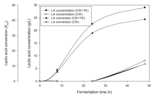
Figure 7. Lactic acid fermentation by L. delbr. subsp. lactis DİSTAM (YE: 0.4% (w/v), ILC: 71.3 g/L, T= 37°C)
