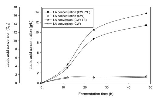
Figure 5. Lactic acid fermentation by L. delbr. subsp. bulgaricus NRRL-B-548 (YE: 0.4% (w/v), ILC: 69.1 g/L, T= 37°C)
