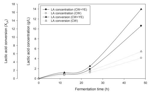
Figure 6. Lactic acid fermentation by L. delbr. subsp. delbrueckii NRRL-B-763 (YE: 0.4% (w/v), ILC: 63.4 g/L, T= 37°C)
