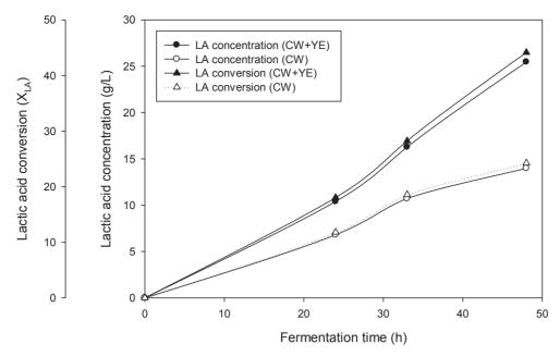
Figure 3. Lactic acid fermentation by Lc. lactis NRRL-B-23802 (YE : 0.4% (w/v), ILC: 57.6 g/L, T= 37°C)
