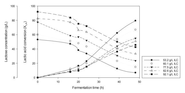
**Figure 8.** Effect of substrate (LACTOSE) concentration on lactic acid conversion and lactose consumption by *Lactobacillus casei* NRRL-B-1922 (YE: 0.4%; ILC: 53.2 g/L, 60.1 g/L, 77.5 g/L, 82.6 g/L, 92.1 g/L, T= 28°C)
