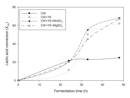
Figure 9. Effect of nutrient supplement on lactic acid conversion by L. casei NRRL-B-1922 (YE: 0.4%, ILC: 57.7 g/L, T=28°C)
