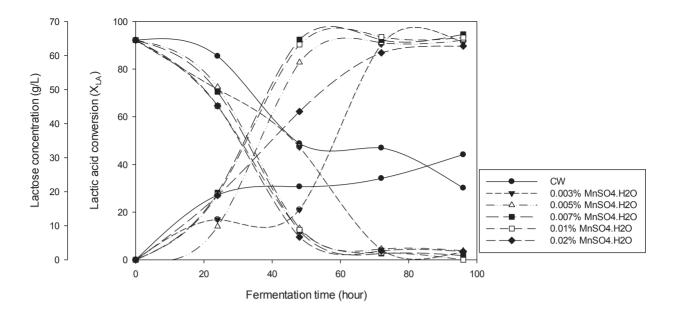
Figure 11. Effect of  $MnSO_4$ ,  $H_2O$  amount on lactic acid conversion and lactose consumption by *Lactobacillus casei* NRRL-B-1922 (YE: 0.4% (w/v), ILC: 64.5 g/L, T= 28°C
