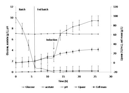
**Figure 4.** A typical time course of exponential fed-batch fermentation using *E. coli* BL21 for lipase production, where the feed medium consisted of a mixture of yeast extract and glucose was used and the required  $\mu$  was set at 0.10 h<sup>-1</sup>.
