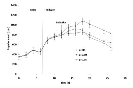
Figure 2. Variation in impeller speed to maintain the DOT at 30 % during exponential fed-batch fermentation conducted with three different required  $\mu$  values.
